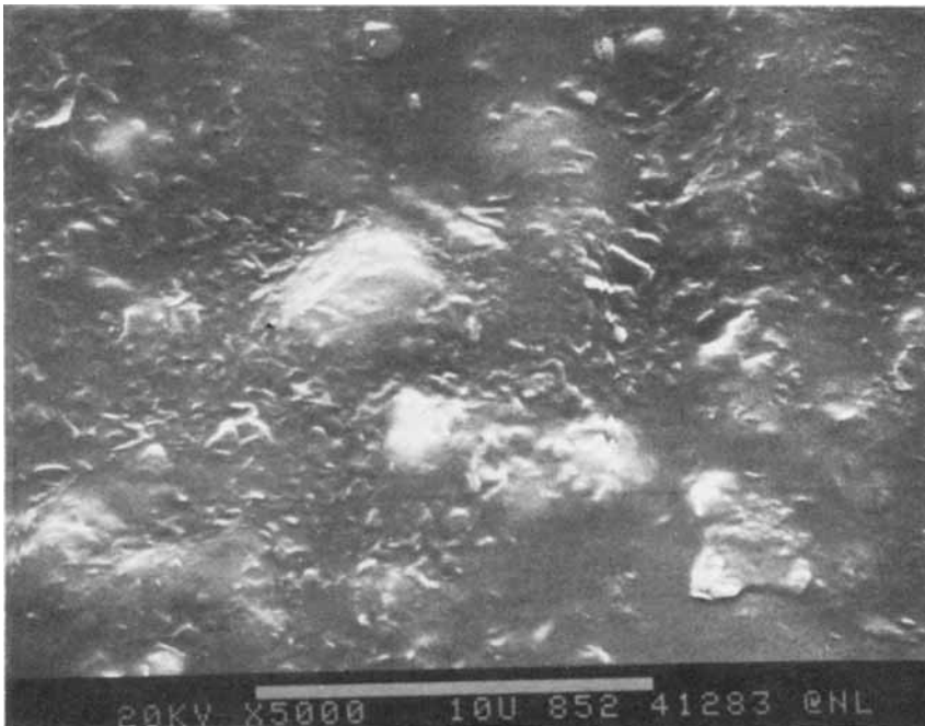
Fig. 15. Surface texture of exposed composite film with S/C 80/20 filler at higher magnification ( \times 2500 ).
